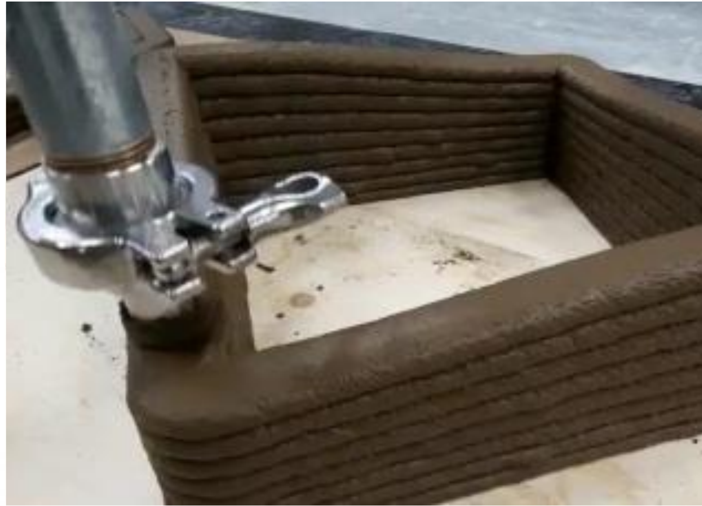
3D-printing with aggregate replacement by regolith simulant
