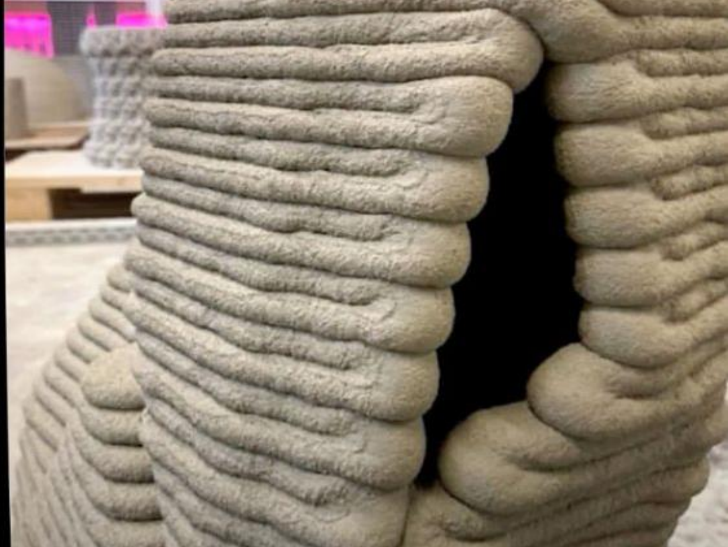
HRI supported assembly of 3D-printed component mock- up
